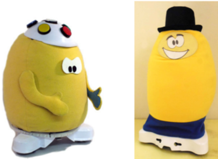
Fig. 1. A first version of Teo, smaller, with cap and velcro-attached eyes, and the final one, with hat and magnetic pad.
